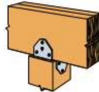
BCS Post Cap: Connects double 2x's to a 4x post or triple 2x's to a 6x post. ZMAX® coating or stainless steel recommended.
