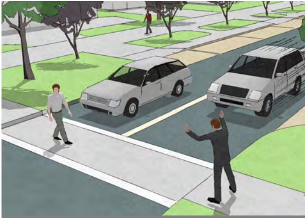
Multiple threat pedestrian conflict
